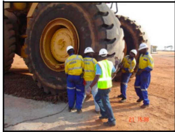
Fig 6. Hooking the chain onto the lug
