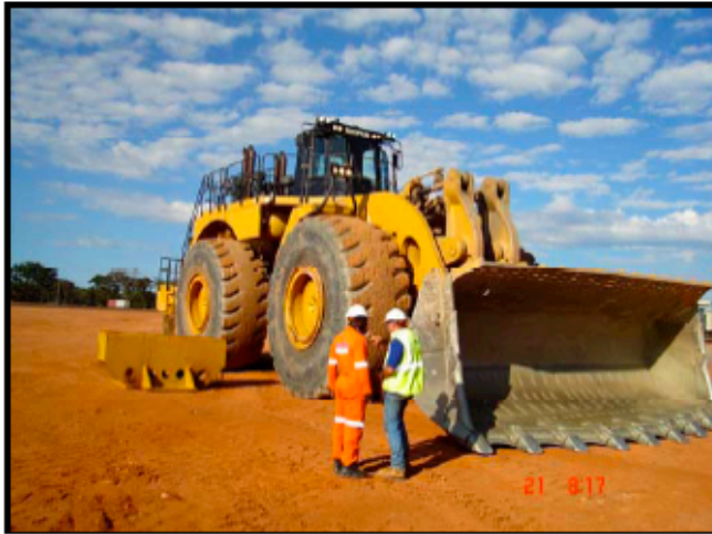
Fig 1. CAT 944F to be fitted with chains. Needed to have a front tyre replaced before fitting chains
