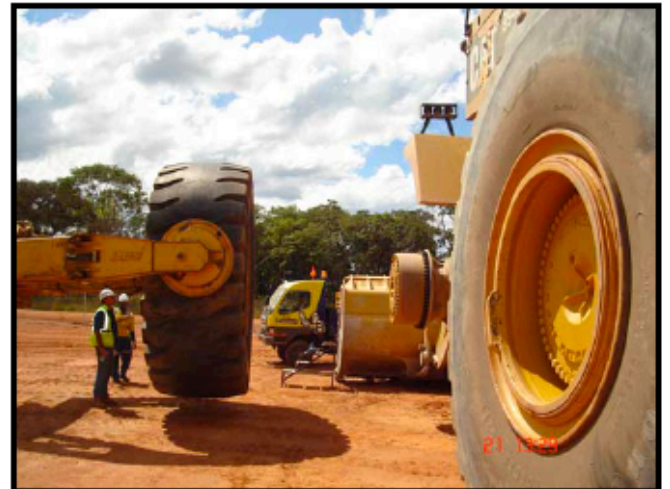
Fig 4. Tyre handling machine lining up to fit new tyre onto hub
